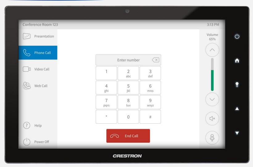
During an active phone call, use the keypad to enter DTMF tones. Press the red *End Call* button to hang up.
