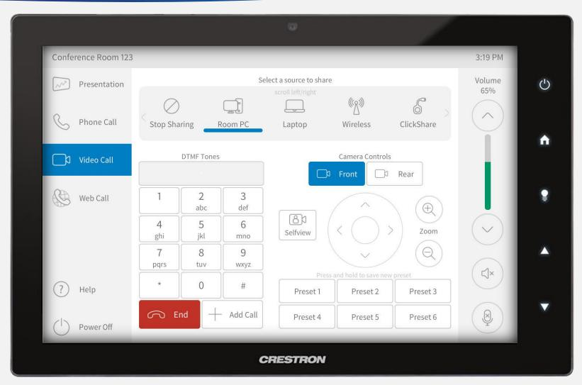
During an active call, select a source at the top of the screen to share with the Far End or press *Stop Sharing* to cease sharing content. Use the keypad to enter DTMF tones and use Camera Controls to position cameras. Press *Add Call* to add call participants. Press the red *End* button to hang up.
