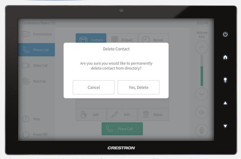
Select a contact then press *Delete* at the bottom of the Contacts screen. A confirmation popup will appear. Press *Yes, Delete* to remove entry from saved contacts.
