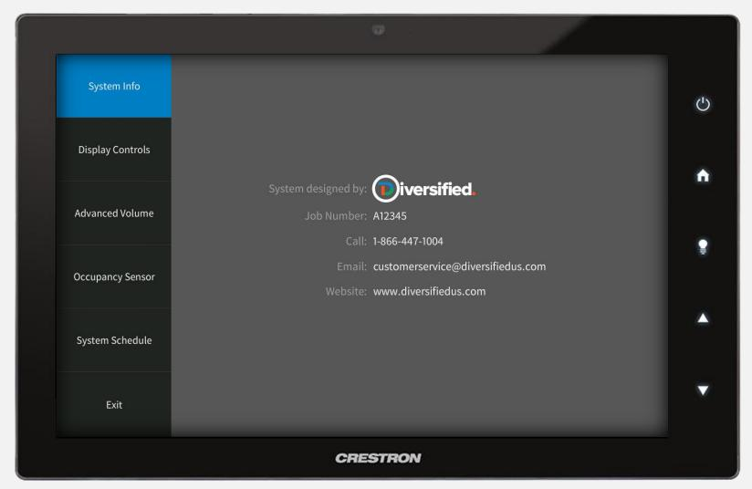
Press and hold the room name in the upper left corner of the Main Page to access the Technician Section. Select *System Info* from the left menu. This screen provides Project and Diversified contact information. Press *Exit* to return to the Main Page.
