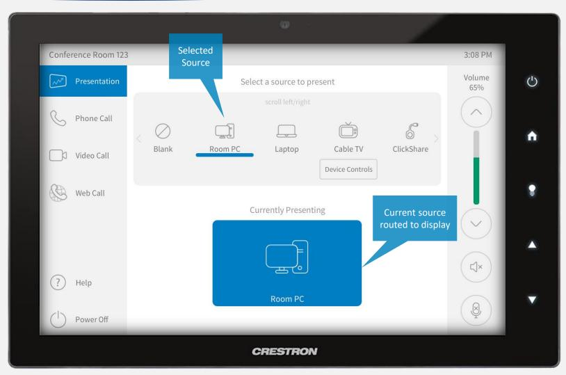
Select *Presentation* from the left menu. At the top of the screen select a source and it will be routed to the room display. Select *Blank* to clear the route to the display. Press *Device Controls* under a source to access additional source controls.
