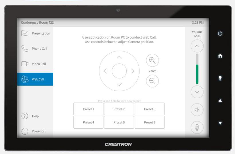
Select *Web Call* from the left menu. Use application on Room PC to start and conduct call. If the system allows for it, use the controls on touch panel to adjust camera position.
