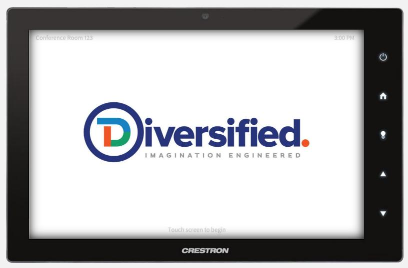
The Splash Screen is visible when the system first boots up or is currently inactive. Touch anywhere on the screen to wake up the system and proceed to controls.
