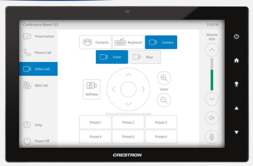
Select *Video Call* from the left menu. At the top of the screen, select *Camera*, then below select either the *Presenter* or *Audience* Camera to control. Use the up/down/left/right and Zoom in/out buttons to adjust camera position, or select a preset at the bottom of the screen to recall. To save a new preset, press and hold a preset button.
