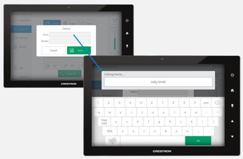
Press *Add* or *Edit* at the bottom of the Contacts page and a popup will appear with text fields for *Name* and *Number*. Tap a text field and a keyboard will appear. Enter the desired information, press *OK* to close the keyboard and then press *Save* to store the new contact information.
