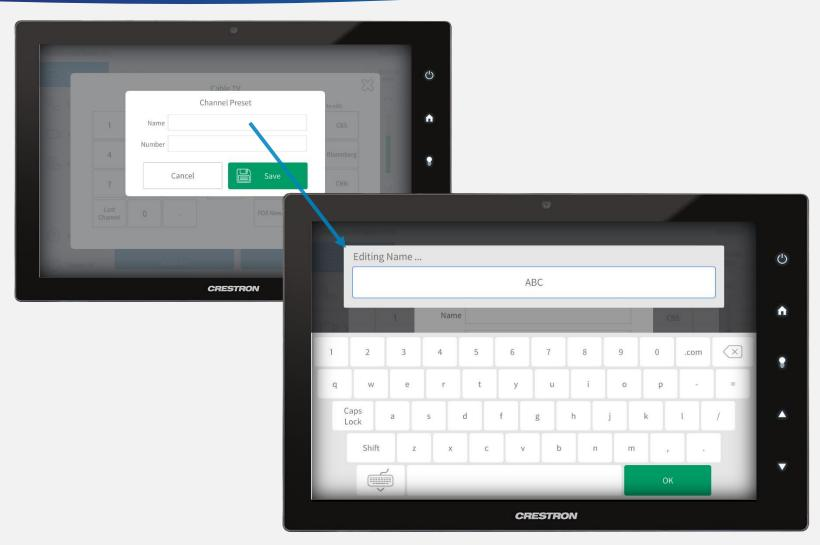
After pressing and holding a channel preset, the *Channel Preset* popup will appear. Tap the *Name* and *Number* text fields to access a keyboard. Enter desired information, press *OK* and to exit keyboard and then press *Save* to store channel preset.
