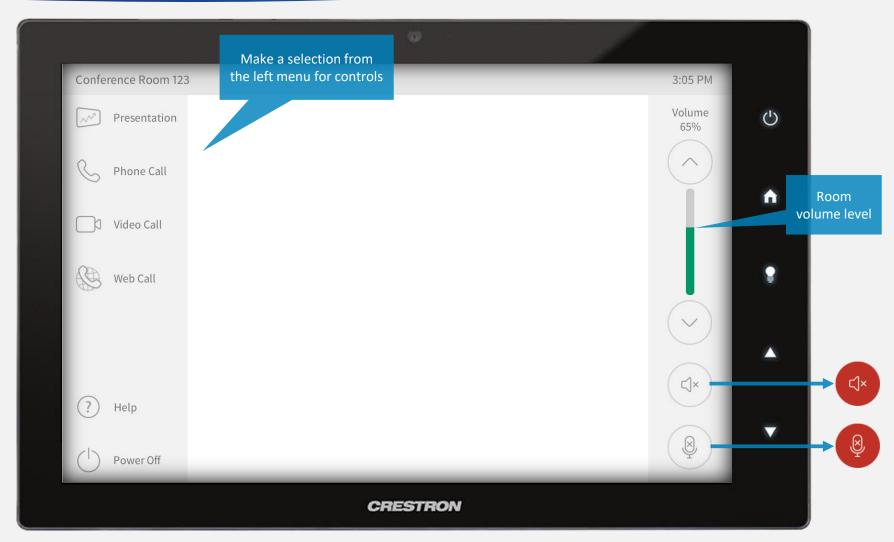
Make a selection from the left menu to access relevant controls. Volume controls are located on the right side of the screen. Use the up/down buttons to adjust room audio. Press the speaker mute icon to mute room audio. Press the mic mute icon to mute all system mics. A muted state is indicated by red. Press again to unmute.
