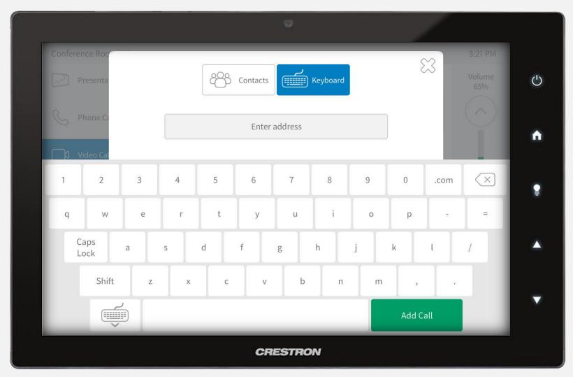
Select Keyboard at the top of the screen and use the keyboard to manually enter an address. Press Add Call to dial.
