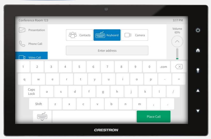
Select *Video Call* from the left menu. At the top of the screen, select *Keyboard*. Use the keyboard to manually enter an address and then press *Place Call* to be connected.
