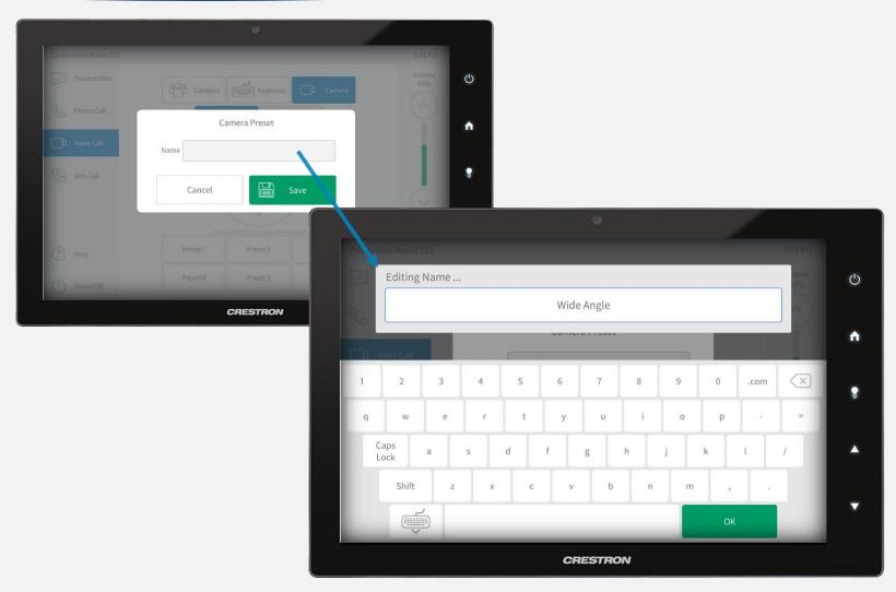
With camera in desired position, press and hold a preset button. A popup will appear. Tap the *Name* text field then use the keyboard to enter desired preset name. Press *OK* to close keyboard, then press *Save* to store new preset.
