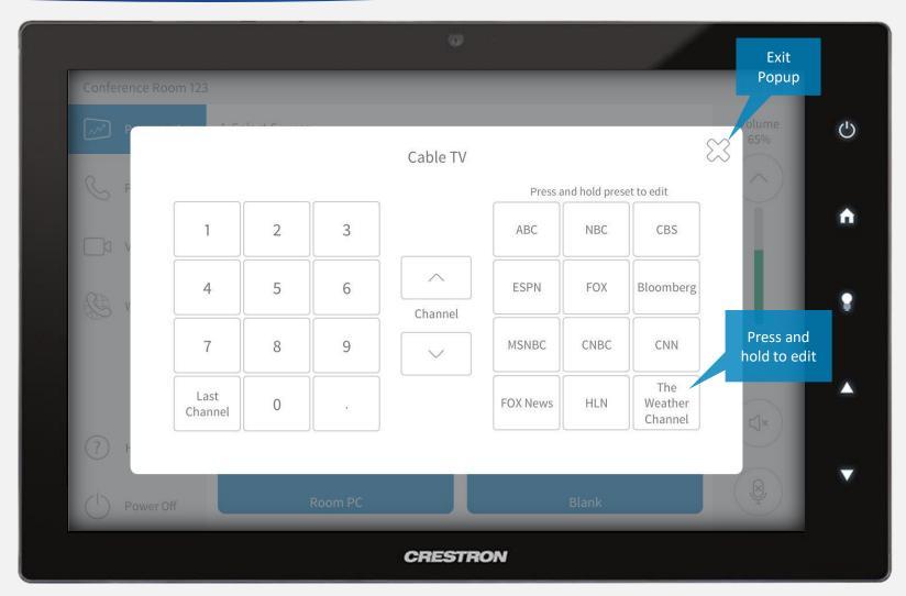
Select *Device Controls* under the Cable TV source to access controls. Use the keypad to enter a channel number, browse channels up/down, or select a channel preset to recall. To edit a channel preset, press and hold a preset button. Press the close icon in the upper right corner to exit.
