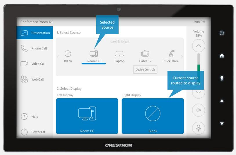
Select *Presentation* from the left menu. At the top of the screen select a source, and then select display(s) in the bottom portion of the screen to route. Select *Blank* and then a destination to clear a route. Press *Device Controls* under a source to access additional source controls.
