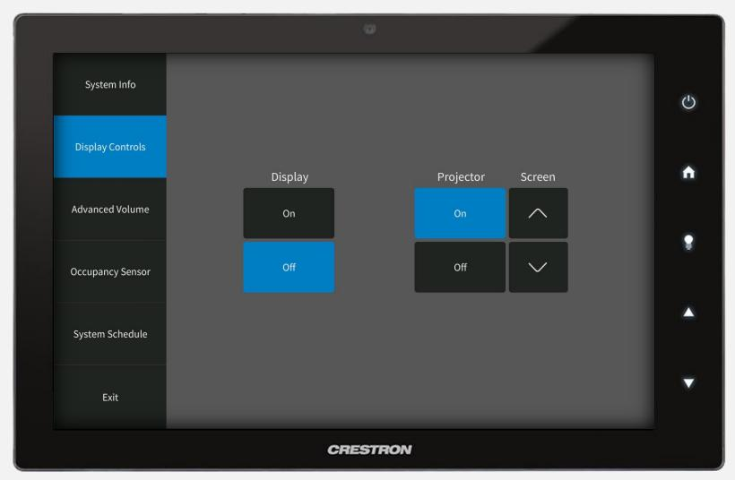
Select *Display Controls* from the left menu. Use the provided controls to turn displays and projectors on/off and raise/lower projection screens.
