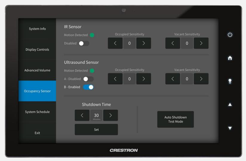
Select Occupancy Sensor from the left menu. Use the provided controls to make various adjustment to sensor settings.
