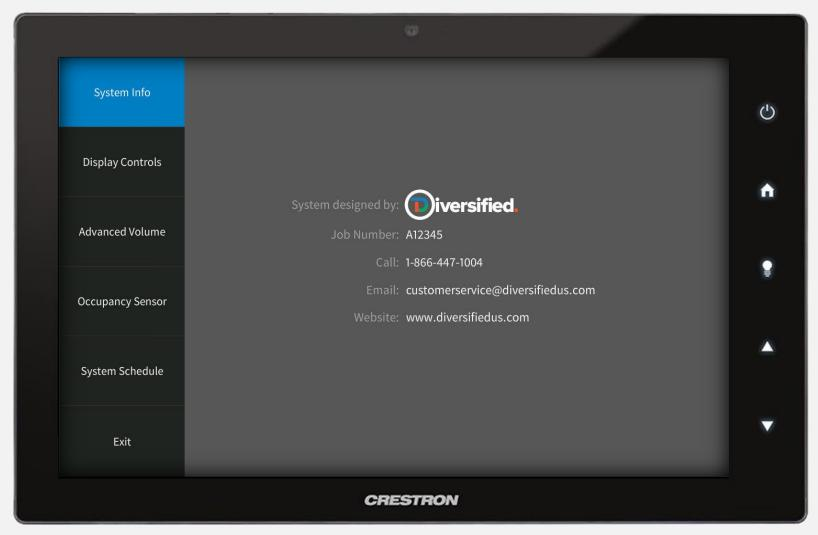
Press and hold the room name in the upper left corner of the Main Page to access the Technician Section. Select *System Info* from the left menu. This screen provides Project and Diversified contact information. Press *Exit* to return to the Main Page.
