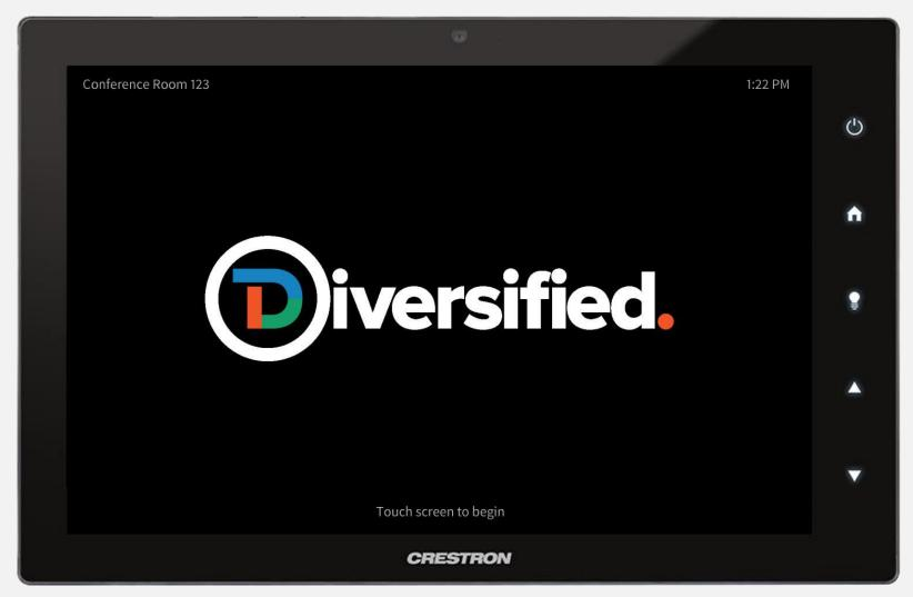
The Splash Screen is visible when the system first boots up or is currently inactive. Touch anywhere on the screen to wake up the system and proceed to controls.
